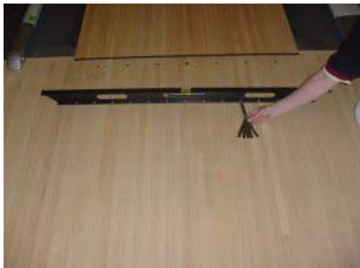
Using Level and Feeler Gauge
